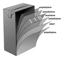
Figure 2. Wall layers of Tetra Pak aseptic packaging.
