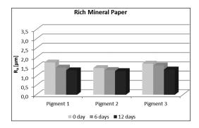
Figure 8: Surface roughness (R<sub>a</sub>) of pearl luster pigments printed on Rich Mineral Paper.
