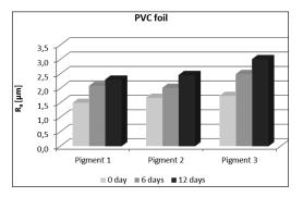
Figure 7: Surface roughness (R<sub>a</sub>) of pearl luster pigments printed on PVC foil.
